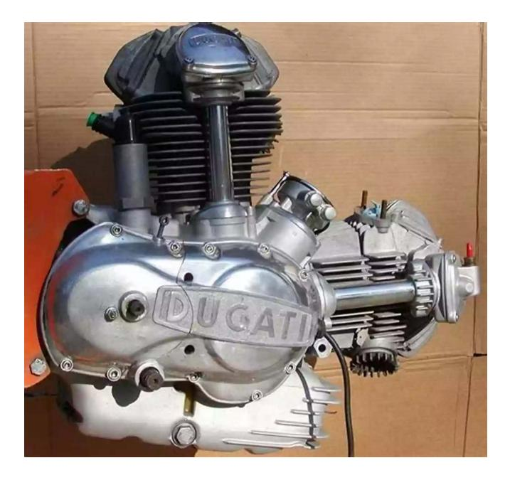
The bike's round case engine, an air-cooled 748cc 90-degree V-twin, showcases Ducati's engineering prowess. This engine layout provided excellent power delivery and a distinct sound that is instantly recognizable on the road. It was accompanied by desmodromic valve actuation, a signature Ducati innovation that eliminated the need for a conventional valve spring system.
